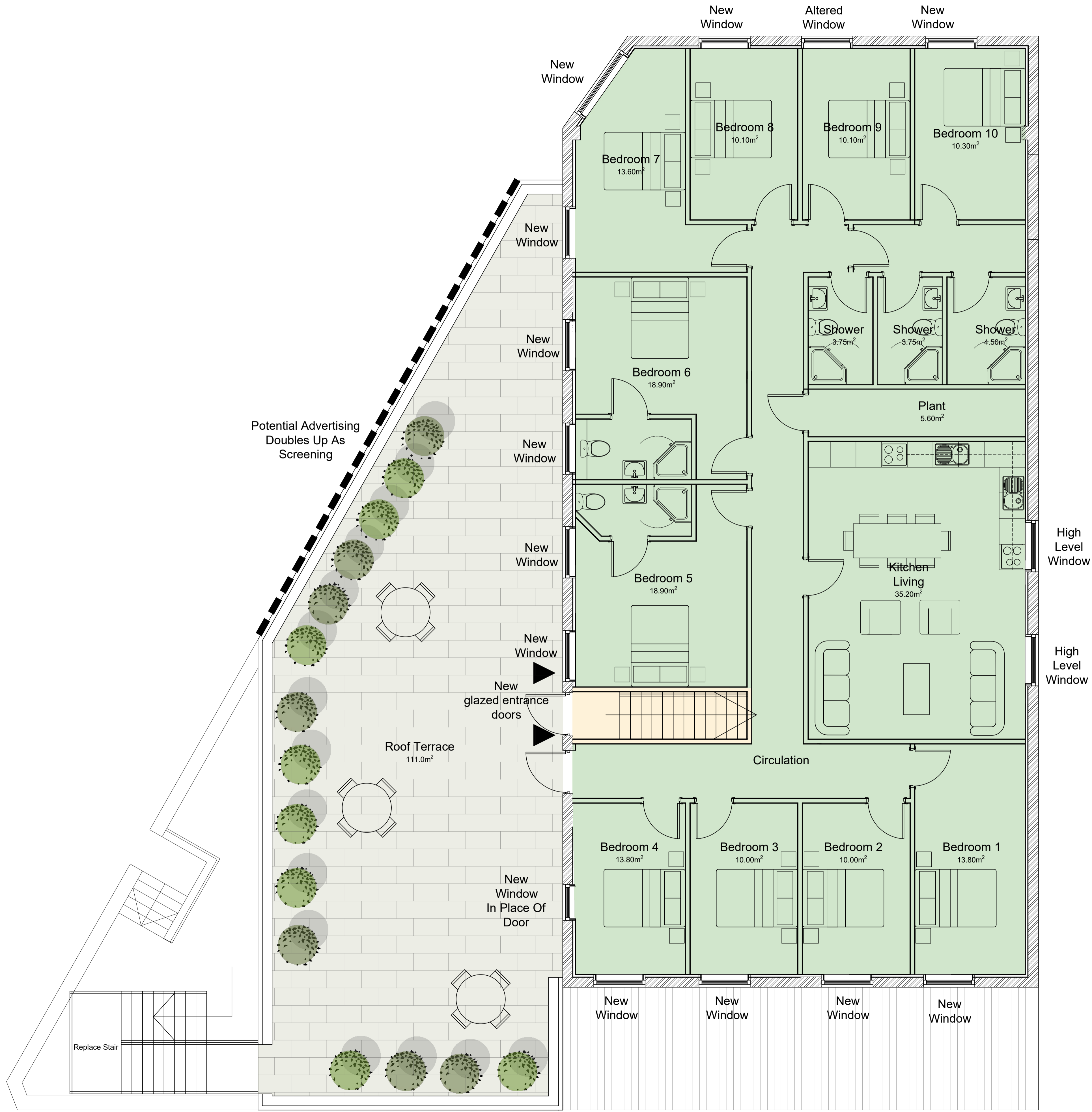
FIRST FLOOR 1:50 External stairs - R:183mm (to be agreed with building control) Levels to be confirmed on site. G: 250mm Min. To be non slip material.
